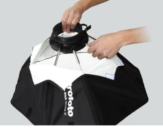
First mount only two rods fully into the speedring (see step 1 and 2), thereafter work yourself around the speedring by mounting the other six rods one by one half way (45 degree angle) into the speedring. Lastly, press the six rods upwards one by one until you hear a click.
