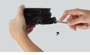
Press the rod upwards until you hear a click, which means the rod is mounted fully into the OCF Speedring.
